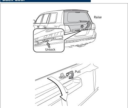
The back door can be locked and unlocked using the entry function, wireless remote control or door lock switch.
